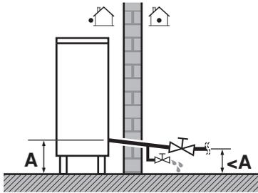
When water is at standstill inside the system, freezing up is very likely to happen and damaging the system in the process.
