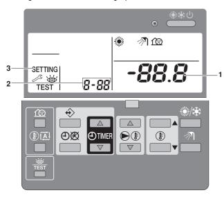
1 Press the substrained button for a minimum of 5 seconds to enter FIELD SET MODE.
