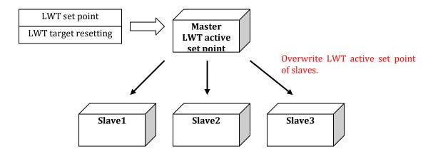
There is one note for calculating return reset. It requires averaged LWT of running units to calculate return reset.
