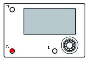
The Remote HMI can be extended up to 700m using the process bus connection available on the UC. With a daisy-chain connection as below, a single HMI can be connected to up to 8 units. Refer to the specific HMI manual for details.
