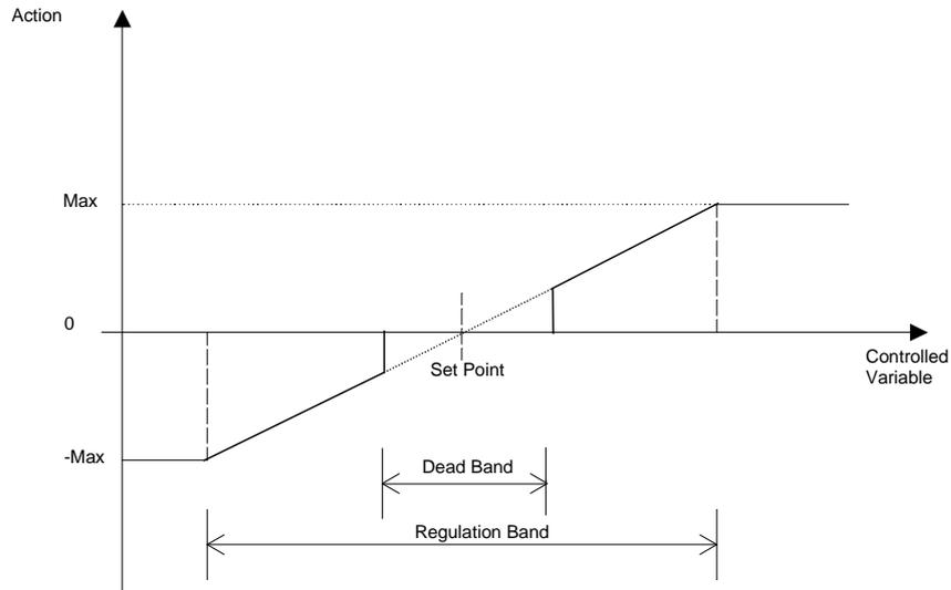
*Fig. 15 – Proportional action of VSD PID in cooling/iced mode*
