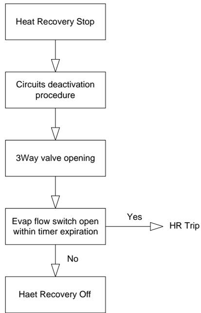
*Fig. 20 – Heat recovery shutdown sequence*
