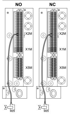
2 Fix the cable with cable ties to the cable tie mountings.
