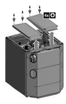
Remove the indoor unit switch box by unscrewing fixations and by then sliding the switch box aside without disconnecting any wiring connections.
