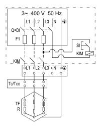
Q\*DI Earth leakage protector (field supply)
