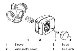
4 Put the sleeve on the valve and turn the valve so that the sleeve is positioned according to the figure below.
