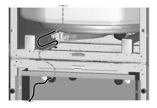
The distance between the thermistor cable and power supply cable must always be at least 25 mm to prevent electromagnetic interference on the thermistor cable.
