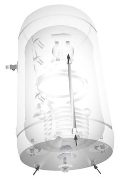
Route the thermistor cable in a conduit to the thermistor inserting tube located above the tank switch box.
