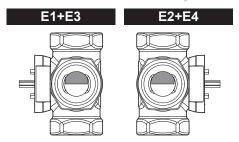
4 When installing in accordance with configurations E3 or E4, open the valve motor cover by loosening the screw and change the jumper so as to change the rotation direction of the valve.
