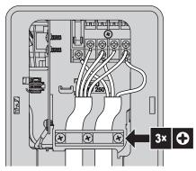
Tighten the terminal screws securely. We recommend using a Phillips screwdriver.
