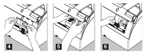
6. Slide the control panel as indicated to attach hooks 1 and 2 to their correct position.
