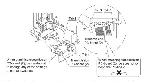
3. Attach the included light receiver assembly (1) to the 2 tabs on the indoor unit, according to following figure.
