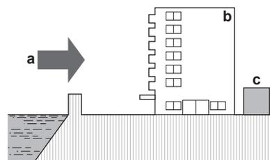
If the outdoor unit is exposed to direct sea winds, install a windbreaker.
